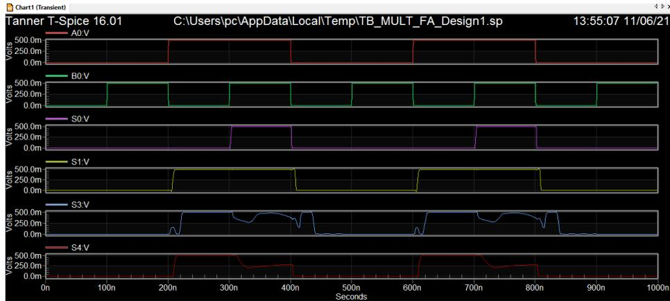
Figure 8 Test bench wave form for the 4-bit MULTIPLIER design
